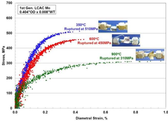
Figure 7: Engineering strain-stress curves of LCAC Mo tested at three different temperatures.
