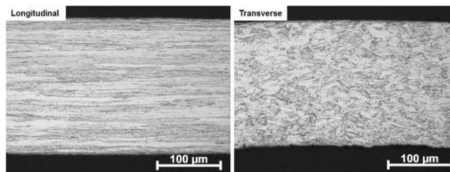
Figure 3: Microstructure of ML tube before induction heat treatment
