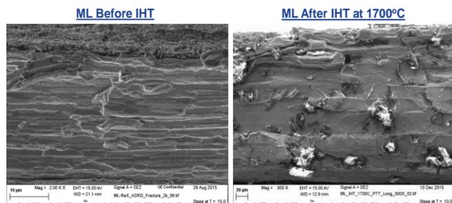
Figure 11: Longitudinal fracture morphology of ML before and after induction heat treatment at 1700°C.
