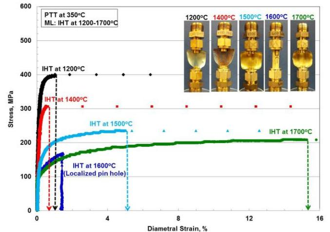
Figure 9: Effect of induction heat treatment at various temperatures on engineering strain-stress curves of ML.
