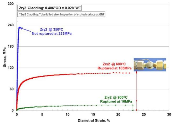
Figure 6: Engineering strain-stress curves for Zircaloy 2 cladding tested at three different temperatures.
