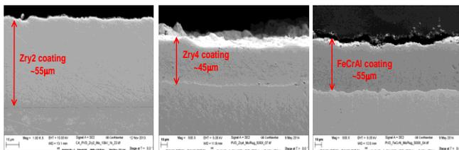
Figure 2: Microstructures of Zircaloy 2 and FeCrAl coating formed by PVD on Mo.
