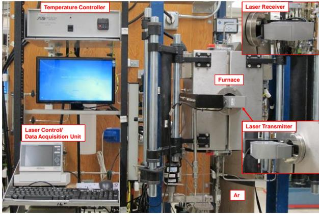
Figure 5: High temperature PTT facility at GEGRC.
