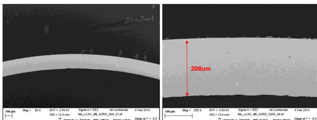
Figure 1: LCAC Mo tube (~8mil wall thickness)
