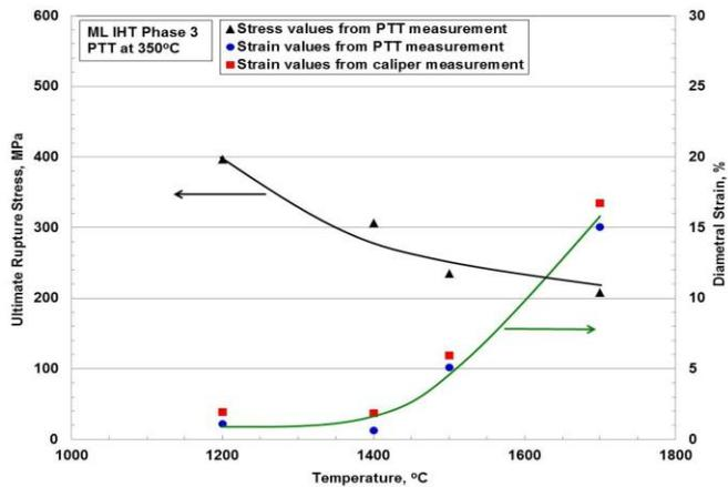
Figure 10: Effect of IHT temperature on rupture stress and diametral strain of ML tube.
