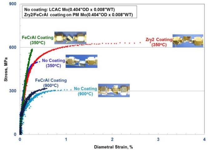
Figure 8: Effect of Zircaloy 2 and FeCrAl coatings on diametral strain-stress curves of LCAC Mo.
