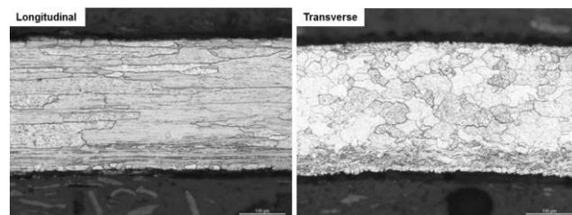
Figure 4: Microstructure of ML tube after induction heat treatment for 5 seconds at 1700°C
