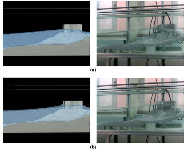
Figure 1. Comparison of simulated and recorded surface motion of the low frequency wave: (a)  $t=8.1s$ ; (b)  $t=8.2s$
