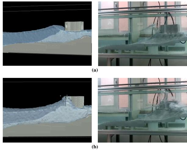
Figure 2. Comparison of simulated and recorded wave for the medium frequency wave: (a)  $t=7.3s$ ; (b)  $t=7.4s$
