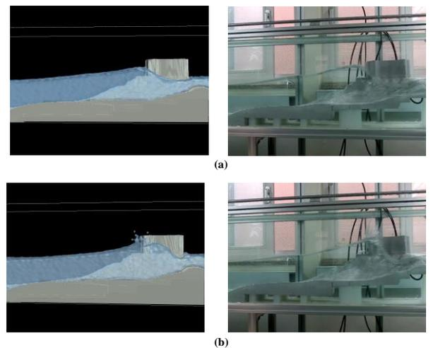
Figure 3. Comparison of simulated and recorded wave for the high frequency wave: (a)  $t=7.0s$ ; (b)  $t=7.1s$
