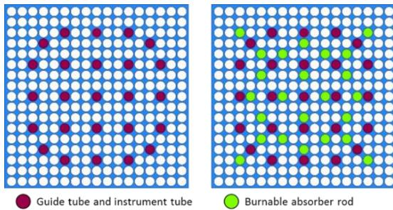
Figure 3. Fuel assembly layout
