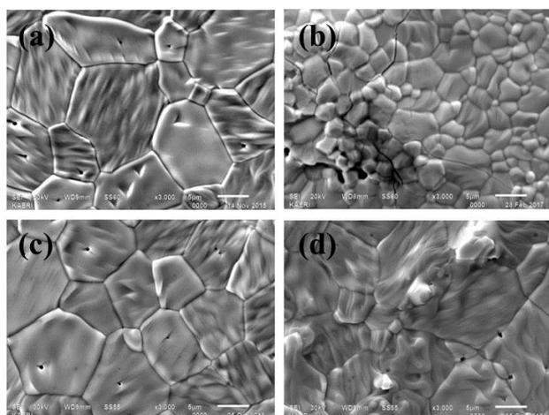
Fig. 1. SEM images of grain structures on the surfaces of (a-b) Zr(IV)-; and/or (c-d) Th(IV)-doped  $\text{UO}_2$ . Doping amounts of each pellets are (a,c) 0; and (b,d) 10 mol%, respectively. Scale bar indicates 5  $\mu\text{m}$  of length.
