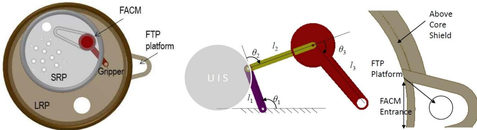
Fig.2 Top view of PG-SFR IVTS
