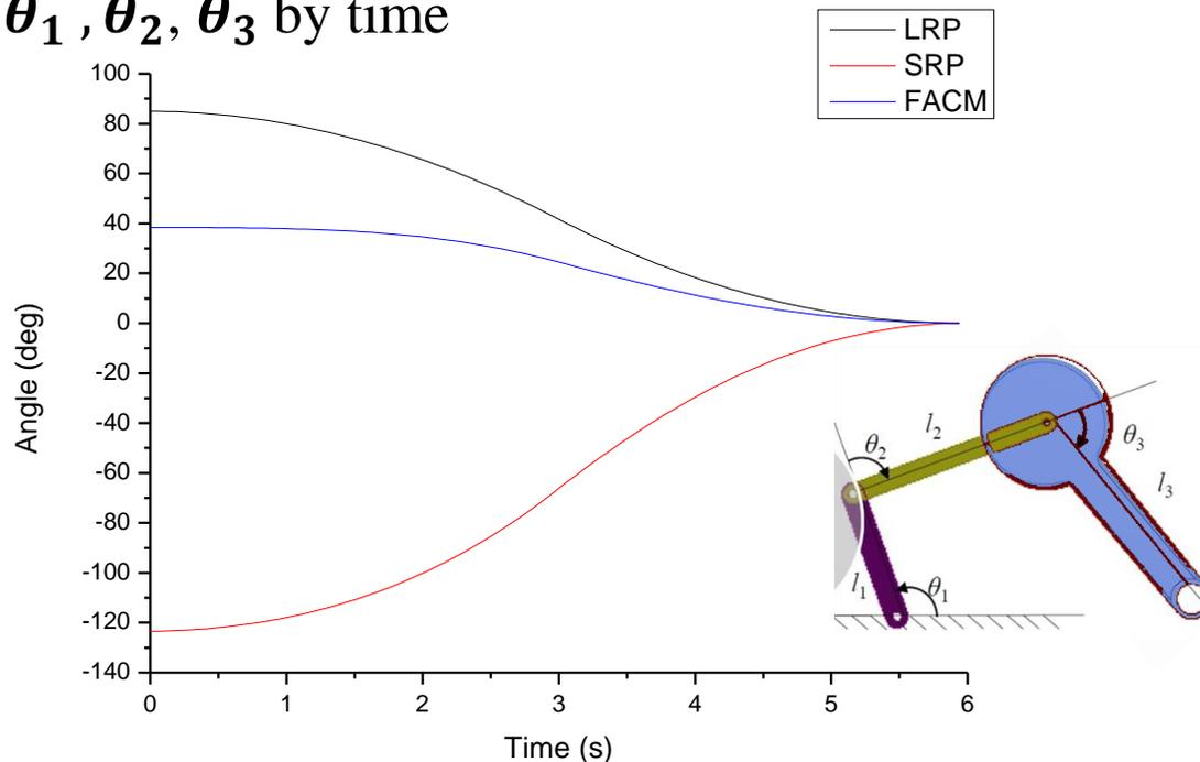
Fig.9 FA Insertion FTP platform ( $V_{avg,LRP} = 2.32 \text{ rpm}$ )
