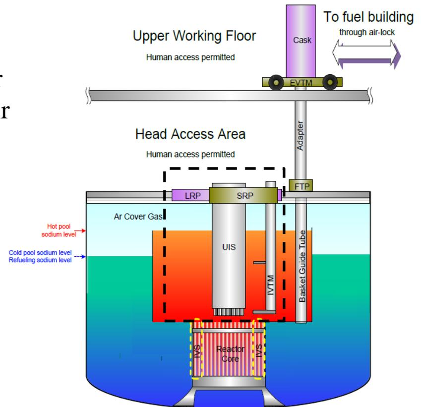
Fig.1 The overview of PGSFR fuel handling with only IVS
