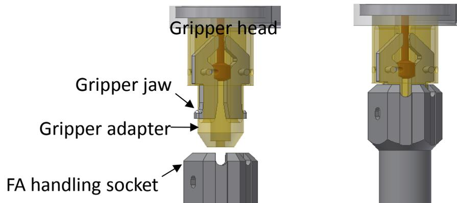
Fig.5 FA gripper in a disengaged view(left), and FA engaged in the gripper (right)
