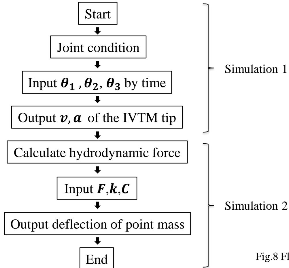
Fig.8 Flow chart of the dynamic simulation
