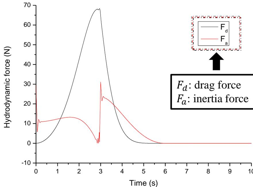
Fig.12 Hydrodynamic forces calculated by the velocity and acceleration
