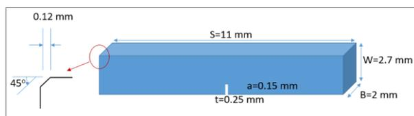
Fig. 4. Sketch of single edge notch beam test sample.
