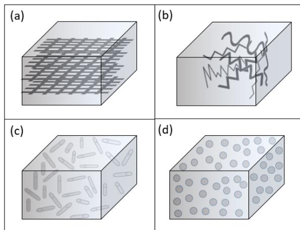
Fig. 1. (a)  $W_{\text{Mesh}}$  (b)  $W_{3D \text{ mesh}}$  and (c)  $W_{\text{Short Fibers}}$  and (d)  $W_{\text{Particles}}$  reinforced HEA ( $WTaTiCrV$ ) composites.
