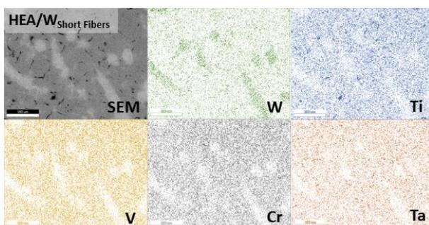
Fig. 3. SEM microstructure and elemental distribution in HEA/W<sub>Short fibers</sub> composite.
