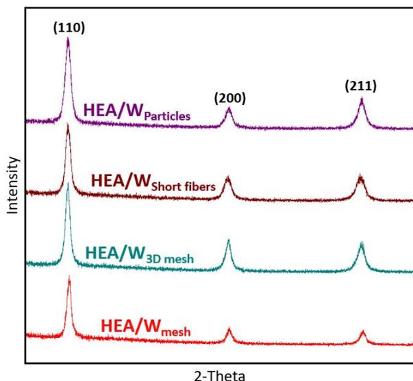
Fig. 2. XRD patterns of W<sub>Mesh</sub>, W<sub>3D mesh</sub>, W<sub>Short Fibers</sub> and W<sub>Particles</sub> reinforced HEA (WTaTiCrV) composites.
