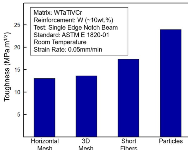
Fig. 5. Effect of various W-based reinforcements on the toughness of HEA/W composites.
