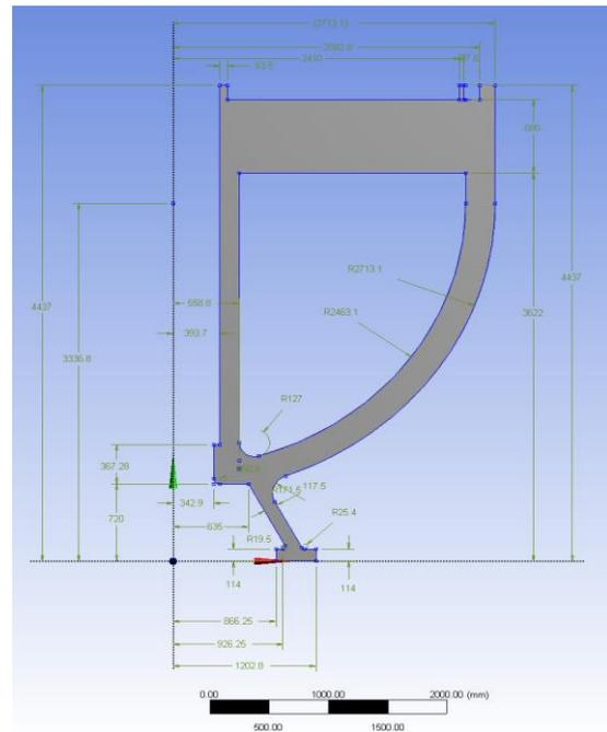
Figure 1 The sketch of the steam generator support
