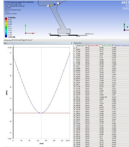
Figure 11 Linearized stress on path 8
