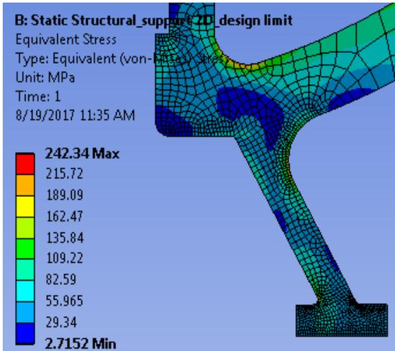
Figure 5 Equivalent stress of the support
