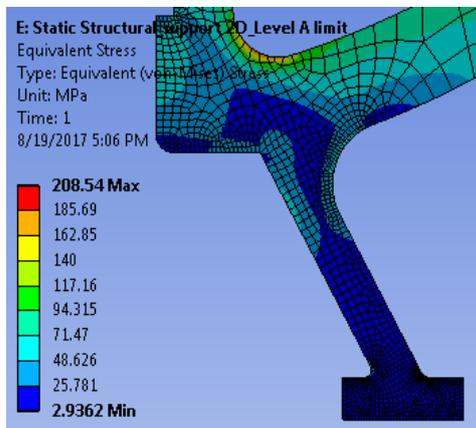
Figure 10 Equivalent stress for level A limits
