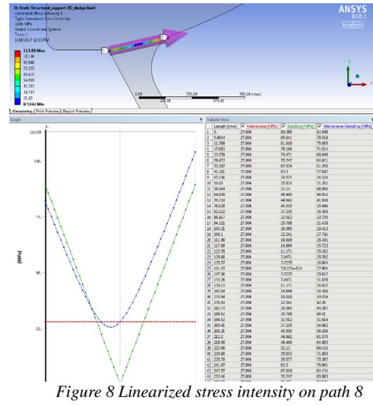
Figure 8 Linearized stress intensity on path 8
