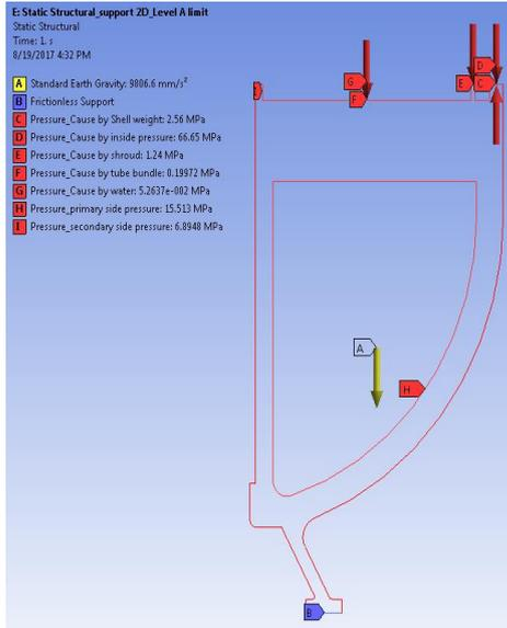
Figure 9 Load combination for level A
