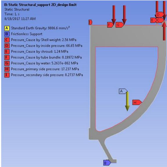
Figure 4 Load combination for design limits
