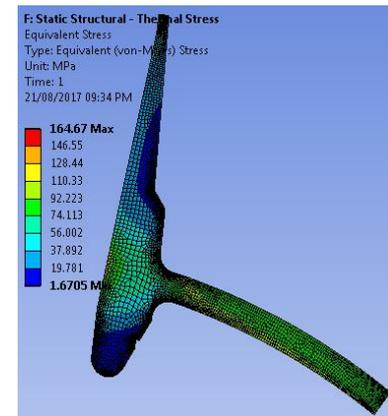
Figure 10: Equivalent stress distribution for full Level A conditions
