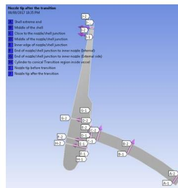
Figure 3: Steam Nozzle stress Path positions 1(A) to 10 (J)
