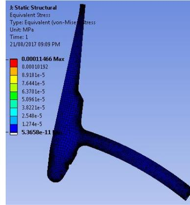
Figure 9: Equivalent stress distribution from thermal gradient
