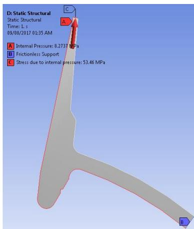
Figure 5: Design loading of the Steam nozzle in ANSYS
