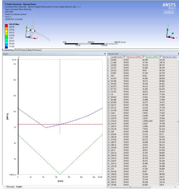
Figure 11: LSI on path 8 at Level A conditions
