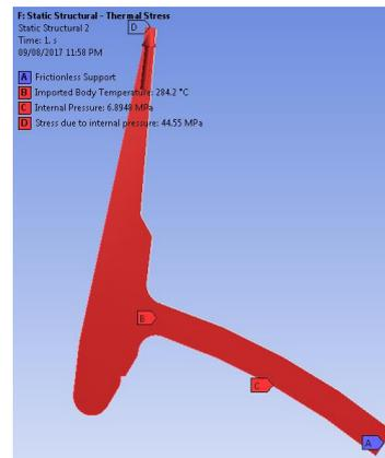
Figure 6: Steam nozzle Level A conditions loading
