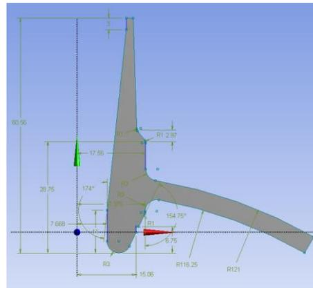
Figure 2: A 2D axisymmetric view of the steam outlet nozzle
