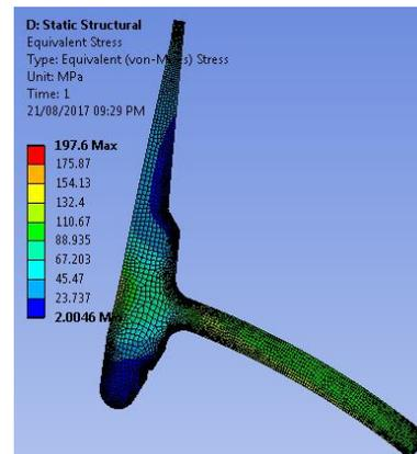
Figure 7: Equiv. stress distribution at design conditions
