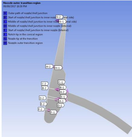
Figure 4: Steam Nozzle stress Path positions 11(A) to 18 (H)
