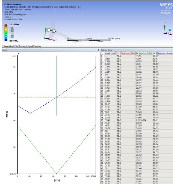
Figure 8: LSI on path 8 at design conditions
