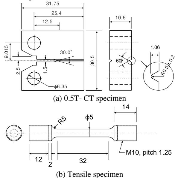
Fig. 1 Specimens used for J-R fracture toughness and tensile tests
