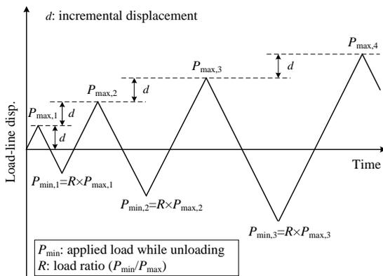
Fig. 2 Loading sequence applied to the cyclic J-R fracture toughness test
