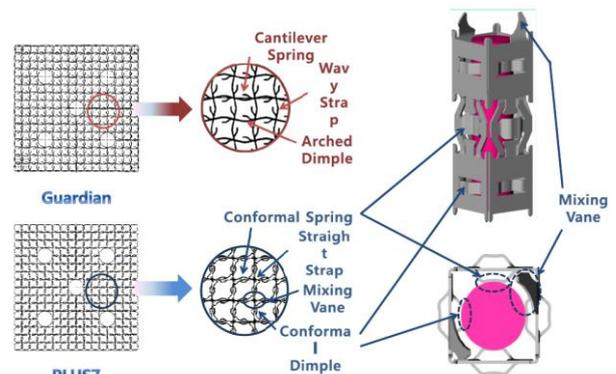
Fig. 2. Difference of Guardian and PLUS7 Fuel Assemblies
