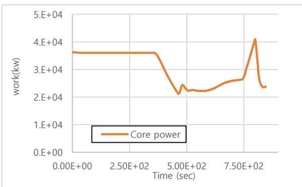
Figure 2.5 MMR core power during ship running simulation
