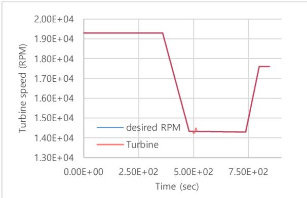
Figure 2.2 Turbine speed during ship running simulation
