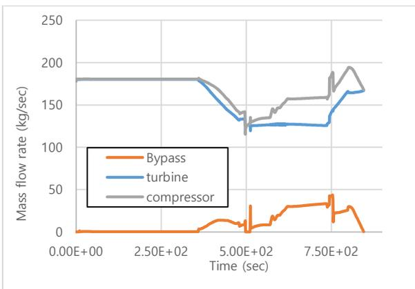
Figure 2.4 Mass flow rate during ship running simulation
