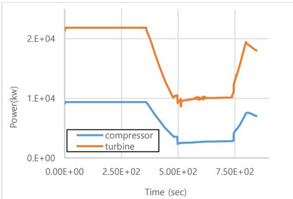
Figure 2.3 Turbomachinery work during ship running simulation
