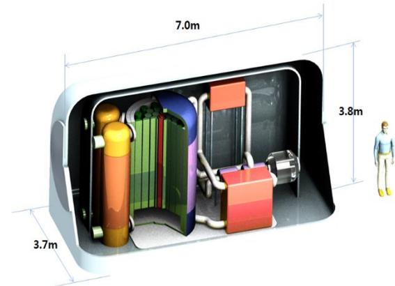
Figure 2.1 Configuration of MMR [6]
