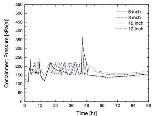
Fig. 2. Comparison of the containment pressure as vent line size (SBO-NE) varies.
