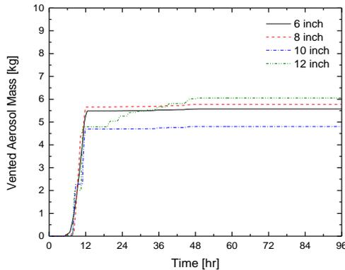
Fig. 4. Comparison of the vented radioactive aerosol masses with varying vent line size (SBO-NE).
