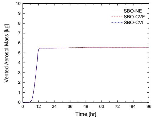
Fig. 1. Comparison of the vented radioactive aerosol mass (SBO-NE, SBO-CVF, and SBO-CVI).
