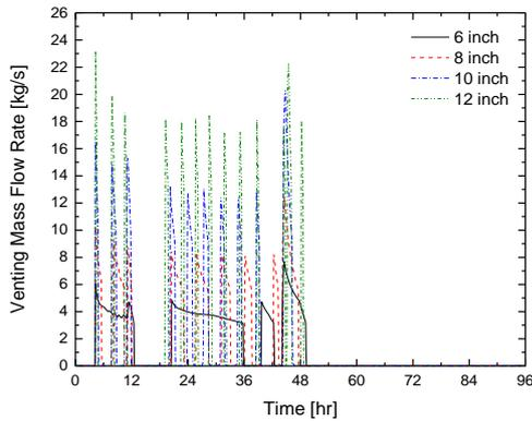
Fig. 3. Comparison of the venting mass flow rates with varying vent line size (SBO-NE).
