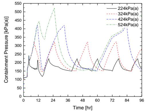
Fig. 5. Comparison of the containment pressures with varying vent initiating pressure (SBO-CVI).
