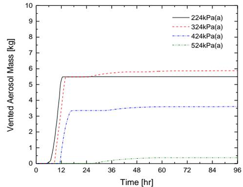
Fig. 6. Comparison of the vented radioactive aerosol masses with varying vent initiating pressure (SBO-CVI).
