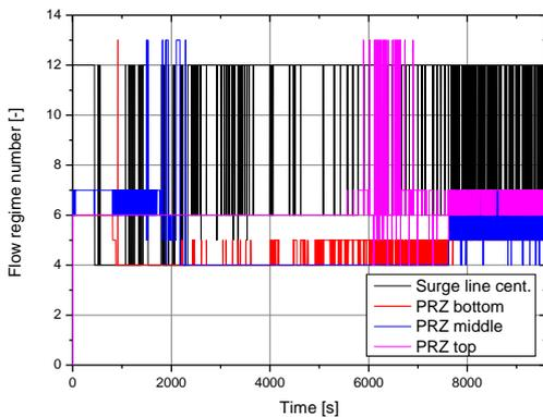
Fig. 4. Flow regime numbers in ML01 (4=bubbly, 5=slug, 6=annular-mist, 7=mist-pre-CHF, 12=horizontal stratified, 13=vertical stratified)
