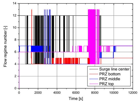
Fig. 6. Flow regime numbers in ML02 (4=bubbly, 5=slug, 6=annular-mist, 7=mist-pre-CHF, 12=horizontal stratified, 13=vertical stratified)
