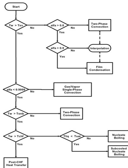
Fig. 3. TRACE wall heat transfer logic diagram for the pre-CHF and condensation regimes [3]
