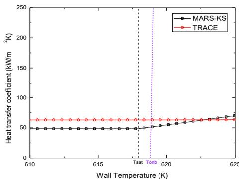
Fig. 6. HTC by  $T_w$  at constant  $T_b$ .
