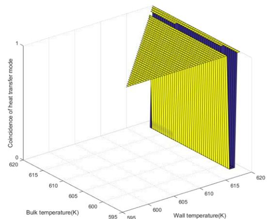
Fig. 4. Similarity of heat transfer mode between MARS-KS and TRACE.
