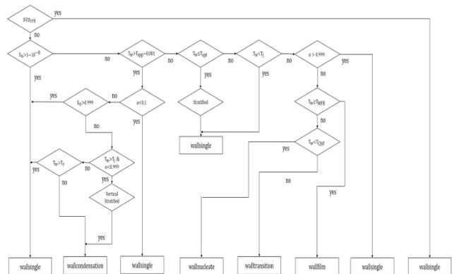
Fig. 2. SPACE wall heat transfer logic diagram [2].
