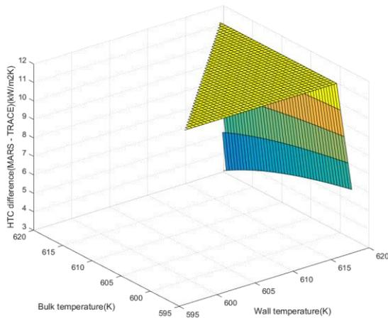
Fig. 5. Difference of HTC between MARS-KS and TRACE.
