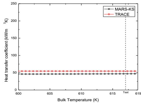
Fig. 7. HTC by  $T_b$  at constant  $T_w$ .
