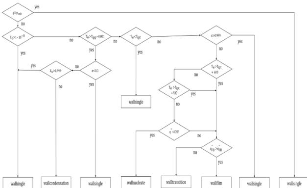
Fig. 1. MARS-KS wall heat transfer logic diagram [1].
