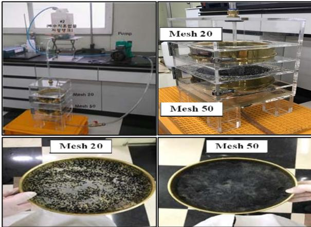
Fig. 4. Spent Resin Mixture Separation System for Simulation (Vertical Structure)
