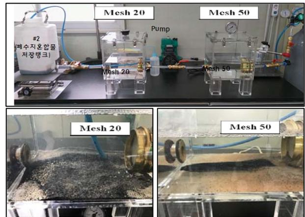
Fig. 3. Spent Resin Mixture Separation System for Simulation (Horizontal Structure)
