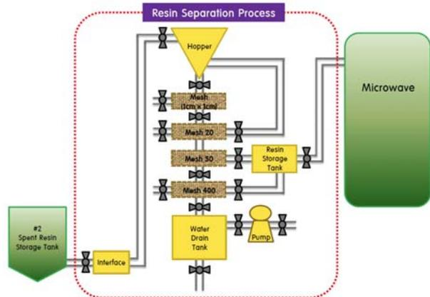
Fig. 5 Resin Separation Process
