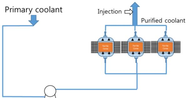
Fig. 4. Primary coolant decontamination process.
