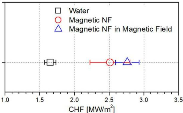
Fig. 3. Magnetic field effect on CHF enhancement.
