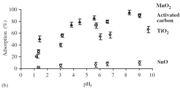
Fig. 10. pH conditions and adsorption rate[4].
