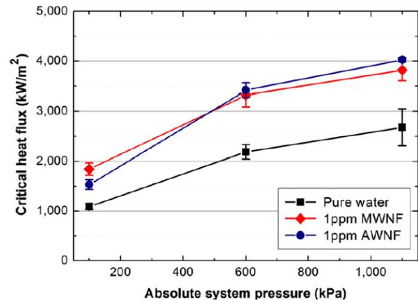
Fig. 6. Pressure effect on magnetic nanofluid.
