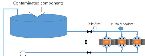
Fig. 5. Components decontamination process.
