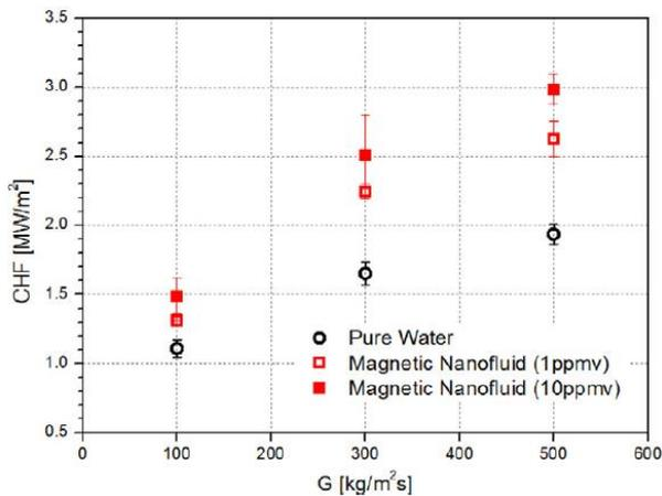
Fig. 2. Magnetic nanofluid used for CHF enhancement where concentration effect is also shown.
