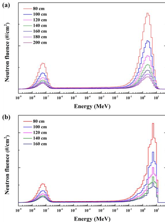
Fig. 2. Neutron fluence spectra at various position from (a)  $^{252}\text{Cf}$  source, and (b)  $^{241}\text{Am-Be}$  source.
