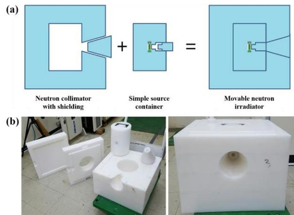
Fig. 1. (a) Concept of packaging for neutron source combined with neutron irradiator, (b) Pictures of movable neutron irradiator combined with neutron source packaging.
