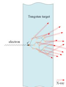
Figure 2. X-ray generation process using tungsten target
