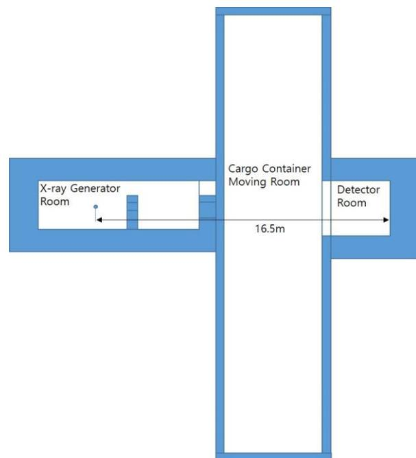
Figure 1. Internal design of container inspection system
