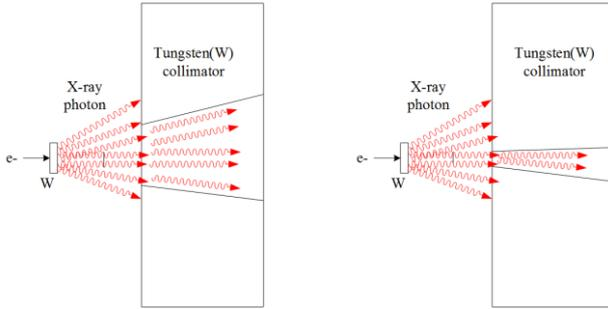
Figure 3. Tungsten collimator model at left and right 0 ~ 4 degrees and up and down -8.5 ~ 15 degree angle for limited angle X-ray beam generation
