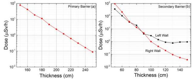
Figure 5. Primary (a) and Secondary (b) Leakage dose surveys according to wall thickness variation
