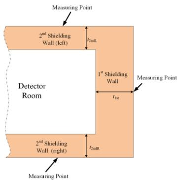
Figure 4. Detector room model for calculating leakage dose using MCNP
