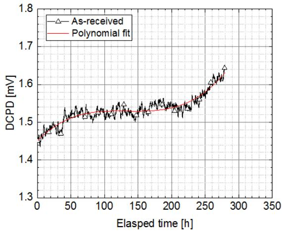
Fig.1 Representative DCPD curve obtained from SSRT.
