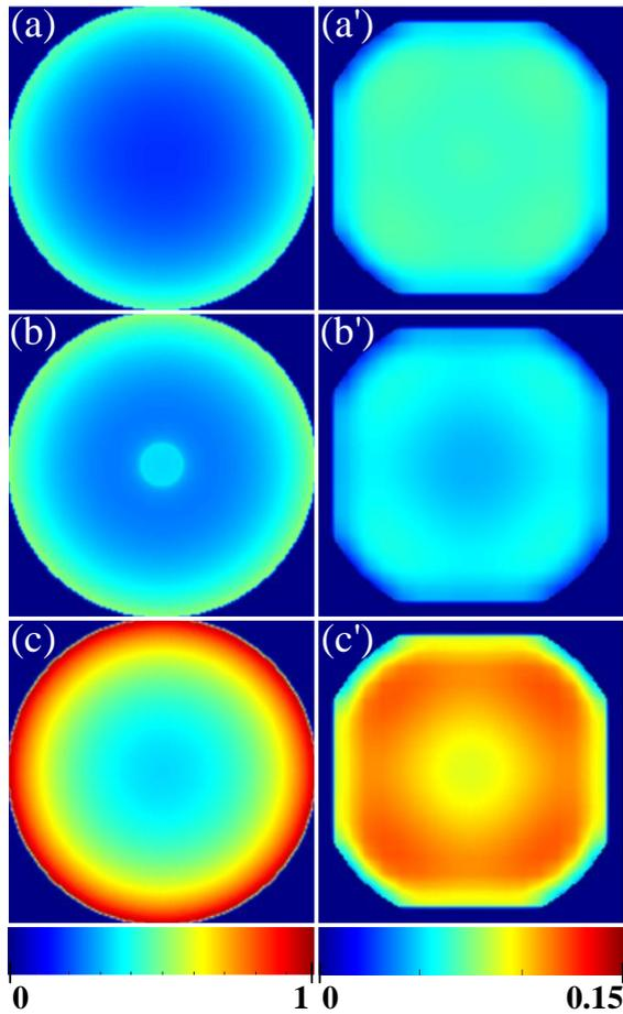
Fig. 2. Absorbed dose in phantom. dose distributions due to the primary and scattered photons. (a) and (a') show primary and scatter dose distributions at half-scan, (b) and (b') at overlapping half-scan, (c) and (c') at full-scan condition respectively.
