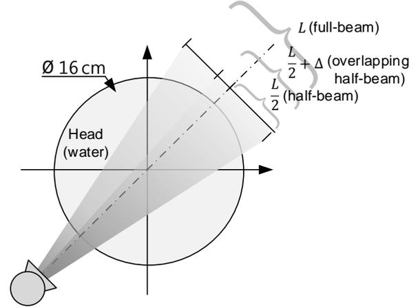
Fig. 1. The phantom and the calculation geometry
