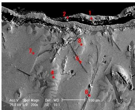
Fig. 4. SEM image of U-10wt%Zr-7wt%RE heel residue.
