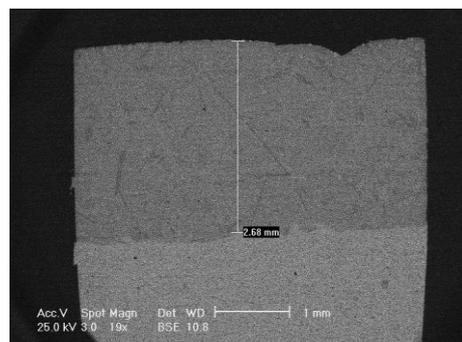
Fig. 2. SEM image of U-10wt%Zr-7wt%RE heel residue.
