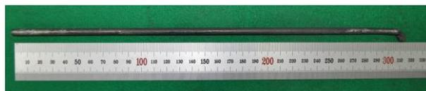
Fig. 5. Recycled U-10wt%Zr-7wt%RE fuel metallic slug.
