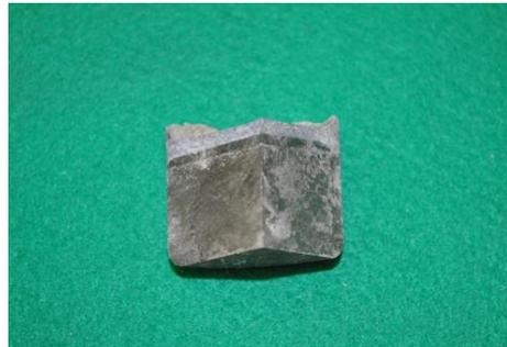
Fig.1. U-10wt%Zr-7wt%RE heel residue.
