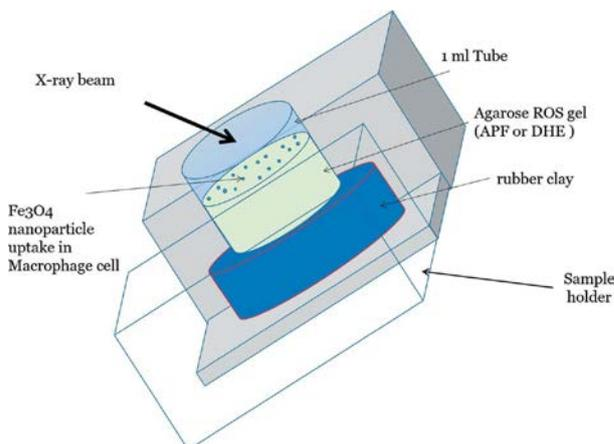
Fig. 1. ROS gel phantom for the measurement of X-ray photoelectric nanoradiator dose.
