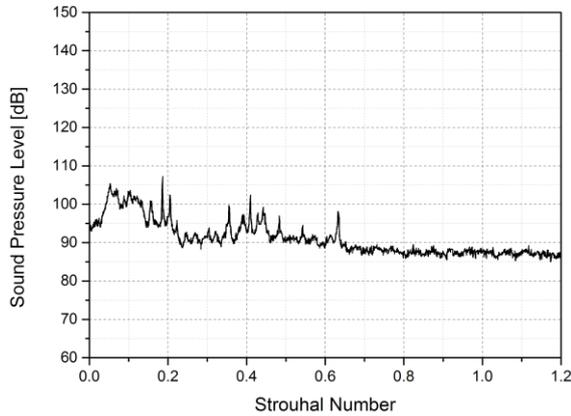
Fig. 7 Jet Impingement Experiment(Thurow, 2002) Result (L/h=8.27)
