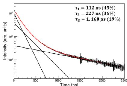
Fig. 5. Decay times of the YAG crystal were measured under  $^{137}\text{Cs}$   $\gamma$ -rays.
