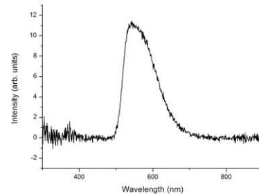
Fig. 3. X-ray induced emission spectrum of the YAG crystal.
