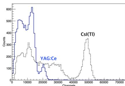
Fig. 4. Relative light yield of YAG and CsI(Tl) crystal for 662 keV from  $^{137}\text{Cs}$  radioactive source.
