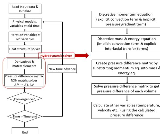
Fig. 1. Algorithm of single phase transient analysis code
