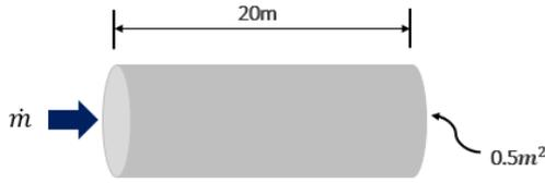
Fig. 2. Configuration of single phase pipe flow with sine pulse of temperature
