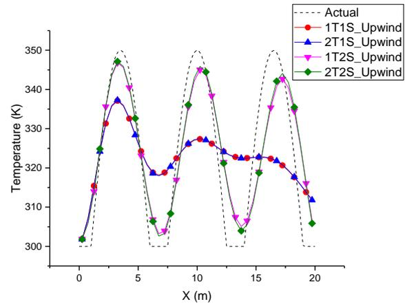
Fig. 5. Sensitivity results of the temporal numerical schemes for the 1<sup>st</sup> order or 2<sup>nd</sup> order upwind scheme
