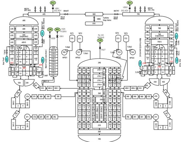
Fig. 1. APR1400 RELAP5 Nodalization Model
