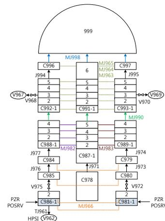
Fig. 2. APR1400 RELAP5 Nodalization Model
