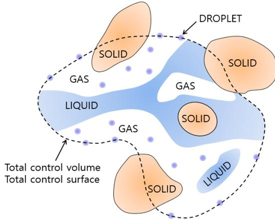
Fig. 1. Gas, continuous liquid, droplet, and solid phases in the total averaging volume.
