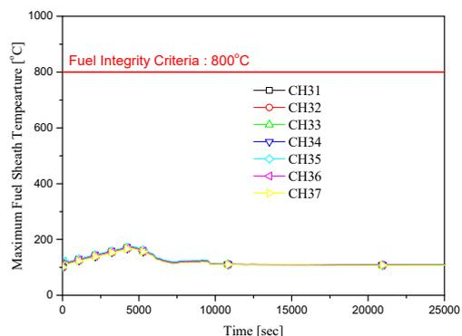
Fig.6. Fuel Cladding Temperature (case B)
