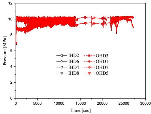
Fig.1. In/Outlet Header Pressure (case A)
