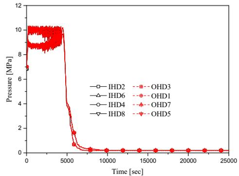
Fig.4. In/Outlet Header Pressure (case B)
