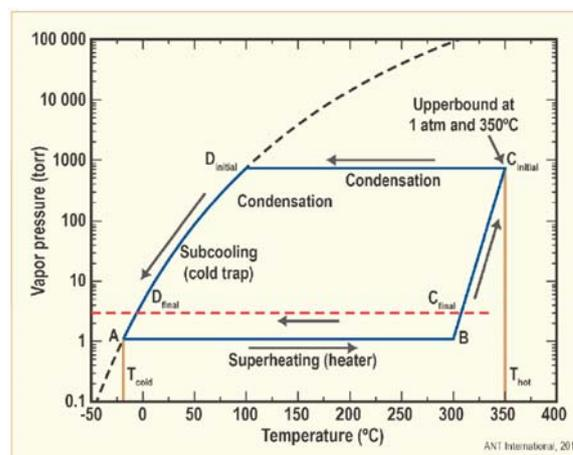
Fig. 3. Pressure–temperature cycle of helium drying process
