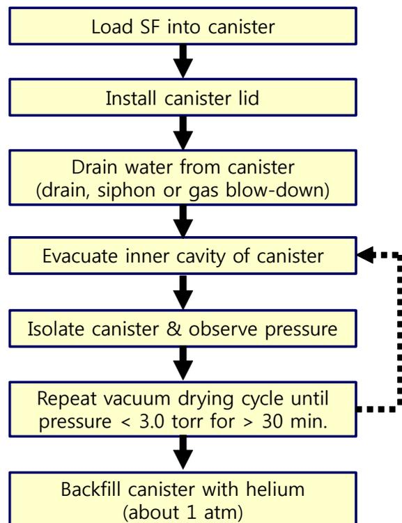
Fig. 1. Flow diagram of vacuum drying process
