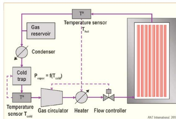
Fig. 2. Flow diagram of forced helium drying process
