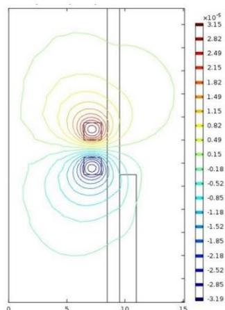
Fig. 2. The distribution of magnetic vector potential of the deposit(1.43 mm height) at the outside surface of the tube.
