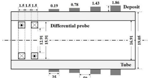
Fig. 1. Parameters in the simulation of eddy current testing for deposits at the outer diameter of the tube.
