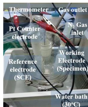
Fig. 5. Photograph of modified DL-EPR cell
