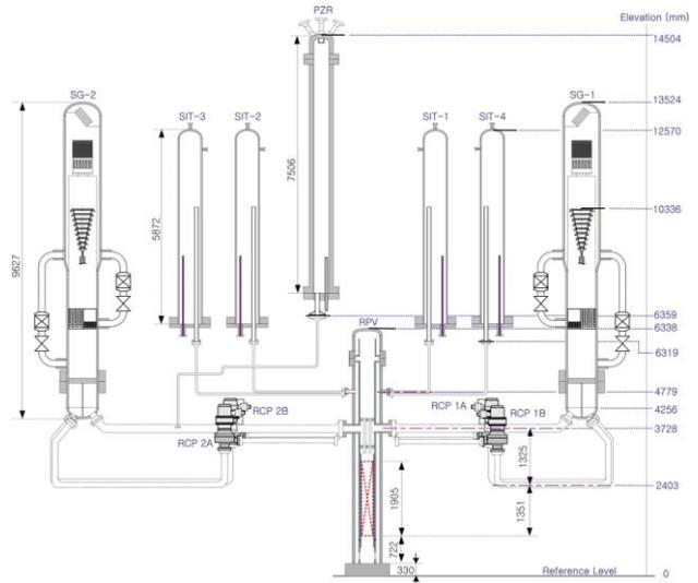
Fig. 1 Schematic diagram of loop connection of ATLAS
