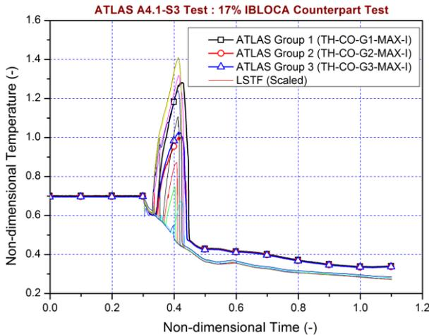
Fig. 5 Maximum heater surface temperature in A4.1 test
