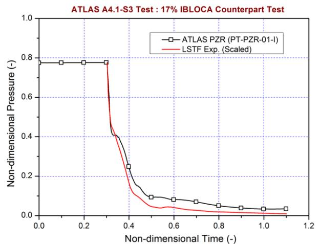
Fig. 3 Primary system pressure in the A4.1 test
