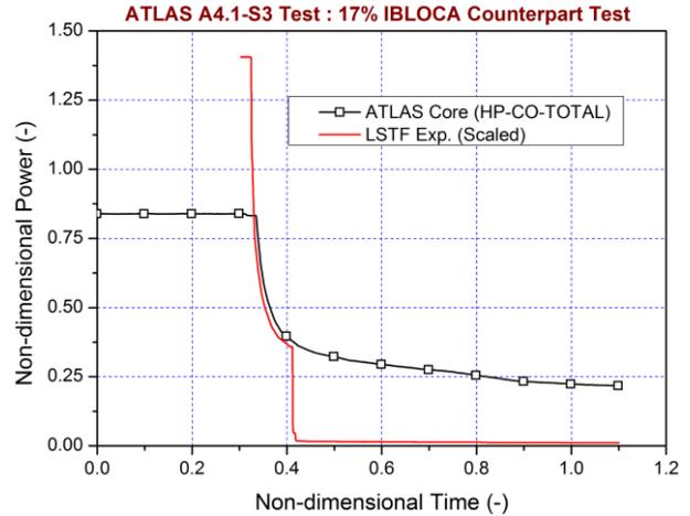
Fig. 2 Core power in the A4.1 test
