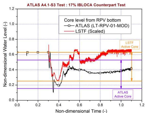
Fig. 4 Core water level in A4.1 test
