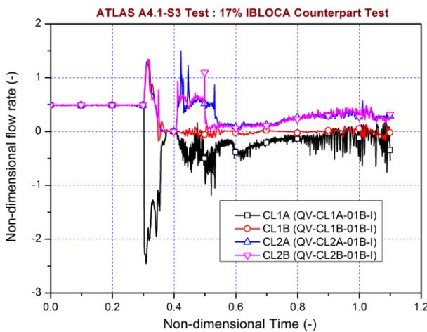
Fig. 6 Cold leg flow rate in A4.1 test
