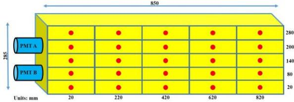
Fig. 2. A 5 × 5 Array in the PVT Scintillator.
