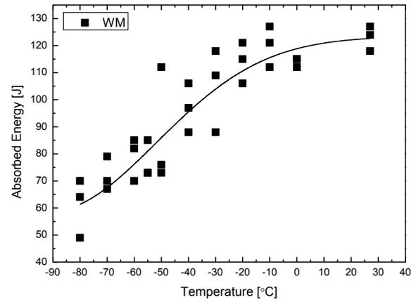
Fig. 3. Results of the Charpy impact test on the WM of the E-beam welding joint after PWHT at 730 °C/1h.
