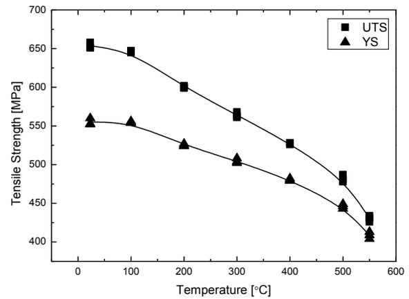
Fig. 4. Results of the tensile strength with temperature after PWHT at 730 °C/1h.
