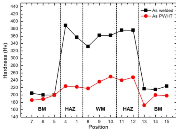
Fig. 1. Results of hardness test across the E-beam welding joint of an ARAA plate before and after PWHT at 730 °C/1h.
