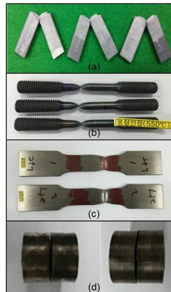
Fig. 5. Results of mechanical property tests (a) Charpy impact test specimens (b) tensile test specimens of dog-bone type (c) tensile test specimens of cylindrical type (d) bend test specimens.
