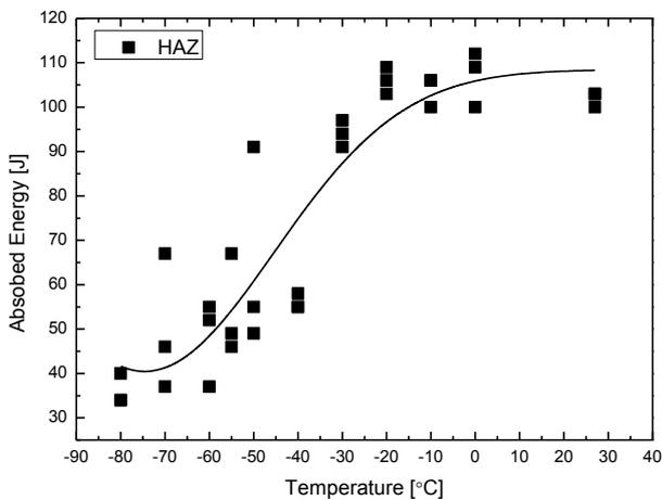
Fig. 2. Results of the Charpy impact test on the HAZ of the E-beam welding joint of an ARAA plate after PWHT at 730 °C/1h.
