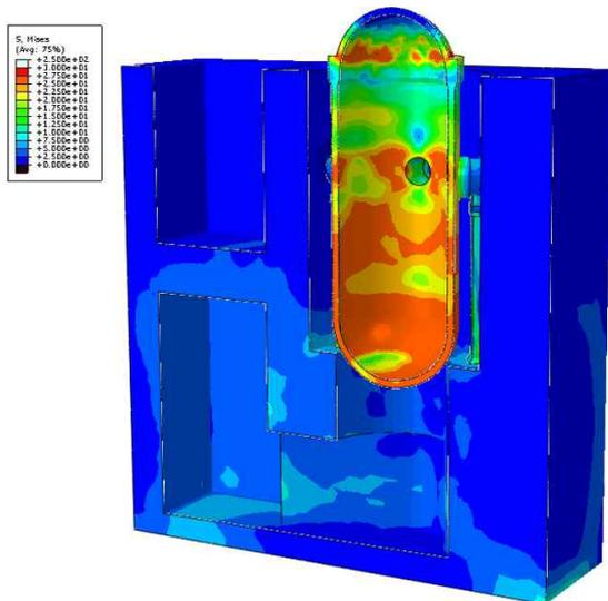
Fig. 2 von Mises stress distribution (Case 3)
