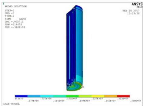
Fig. 4 Stress Distribution for Thermal Stress Analysis
