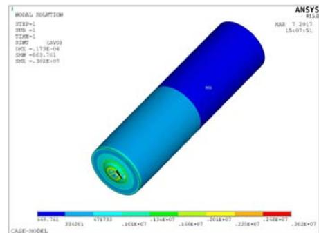
Fig. 2 Stress Distribution for Dead Weight Analysis
