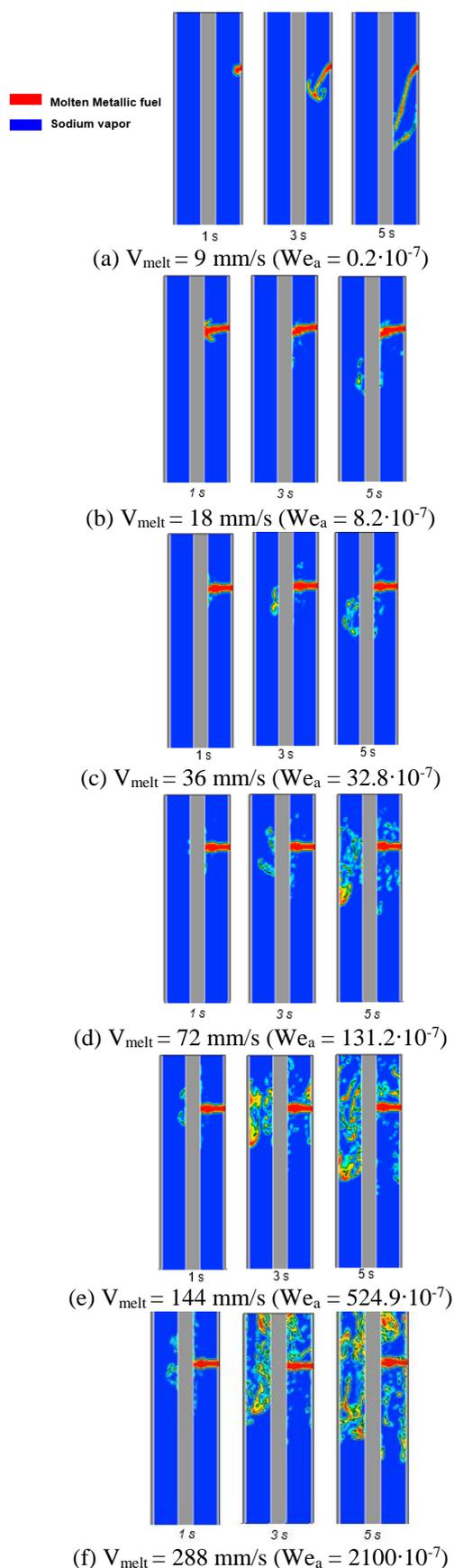
Fig. 3. Behavior of molten metallic fuel in sodium vapor channel
