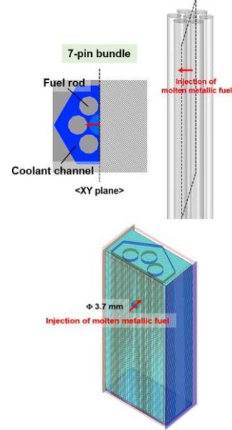
Fig. 2. Grid configuration of CFD model for 7-pin bundle
