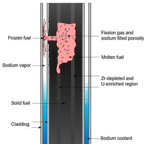
Fig. 1. Configuration of molten fuel behavior during Ex-pin
