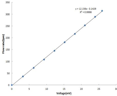
Fig. 3. Volume flow rate versus output voltage from electromagnetic flow meter at 150 °C
