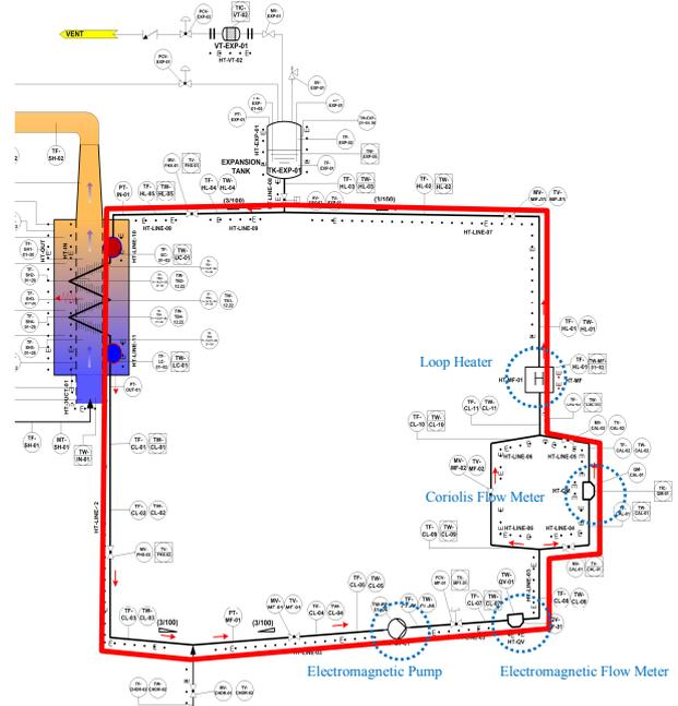
Fig. 2. Flow path for performance test of electromagnetic flow meter
