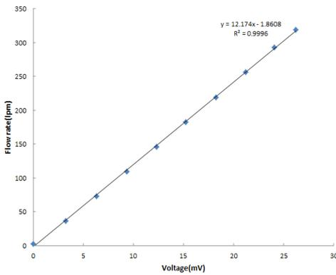
Fig. 4. Volume flow rate versus output voltage from electromagnetic flow meter at 200 °C
