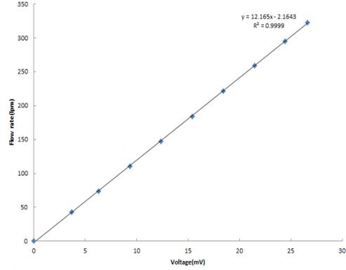
Fig. 5. Volume flow rate versus output voltage from electromagnetic flow meter at 240 °C
