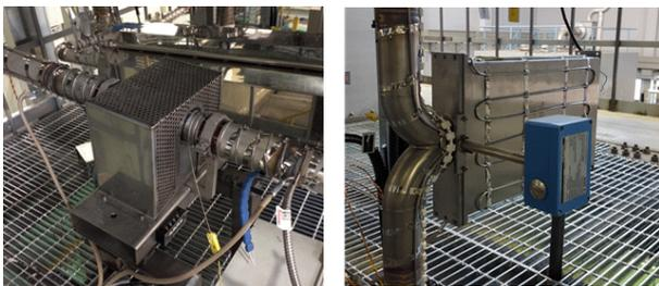
Fig. 1. Electromagnetic flow meter (left) and Coriolis flow meter (right) in the main loop of SELFA
