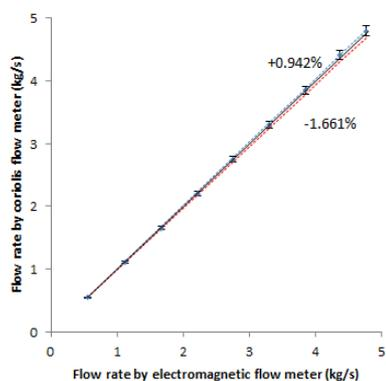
Fig. 7. The percentage of reading accuracy of electromagnetic flow meter versus Coriolis flow meter at 200 °C
