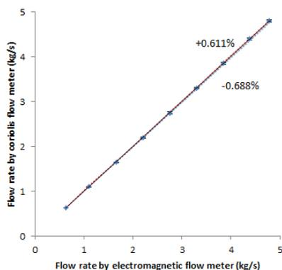
Fig. 8. The percentage of reading accuracy of electromagnetic flow meter versus Coriolis flow meter at 240 °C
