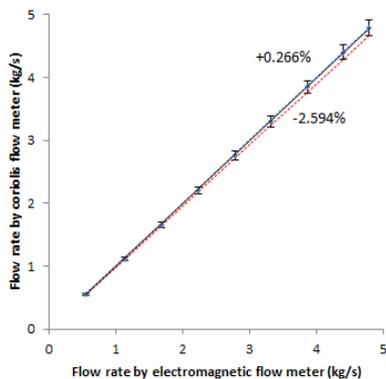
Fig. 6. The percentage of reading accuracy of electromagnetic flow meter versus Coriolis flow meter at 150 °C
