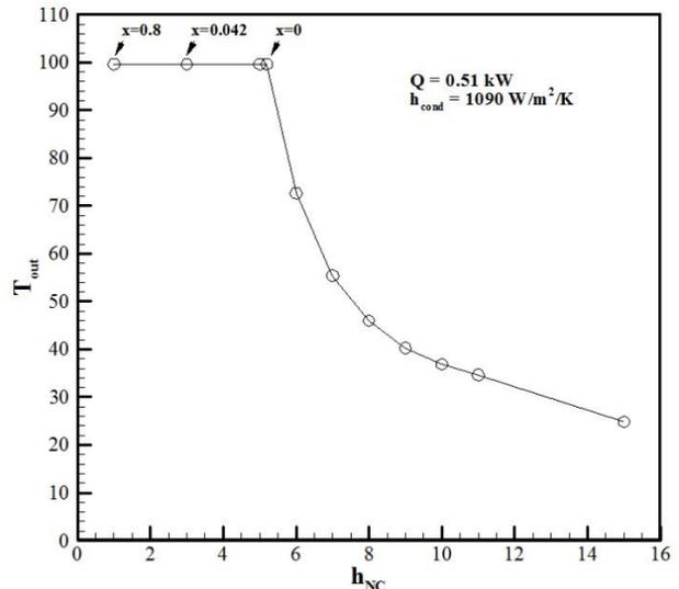
Fig. 5. Outlet temperature vs. average air natural convection coefficient at  $Q = 0.51$  kW and  $h_{cond} = 1090$  W/m<sup>2</sup>/K
