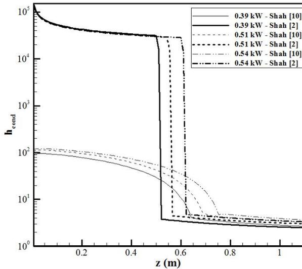
Fig. 3. The comparison of the correlations of condensation heat transfer to the experimental data of Kim *et al.* [1]
