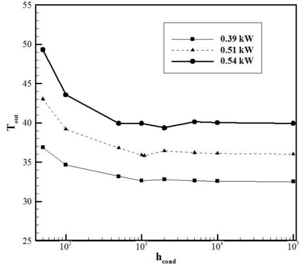
Fig. 4. Outlet temperature vs. average condensation convection coefficient with the experimental data of Kim *et al.* [1]
