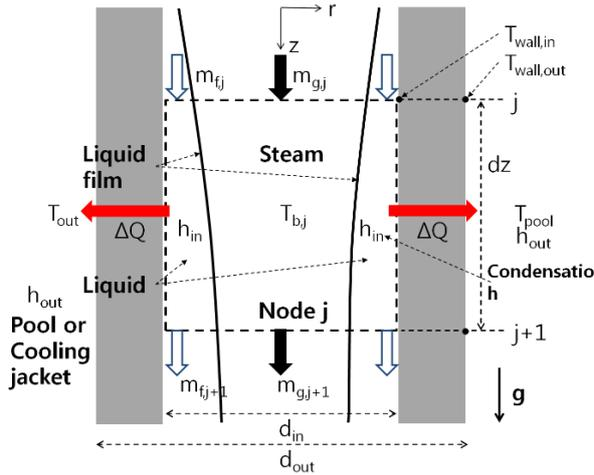
Fig. 1. Schematic of a discretized node of a vertical tube in a condensation heat exchanger [4]
