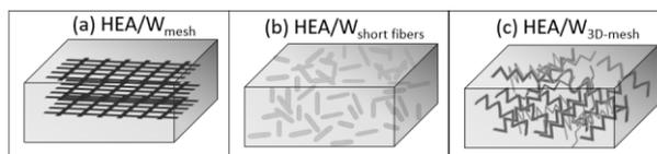
Fig. 1. (a)  $W_{\text{mesh}}$  (b)  $W_{\text{short fibers}}$  and (c)  $W_{3\text{D-mesh}}$  reinforced HEA (WTaTiCrV) composites.
