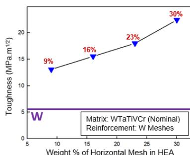
Fig. 4. Effect of weight% of  $W_{mesh}$  on the toughness of HEA composite.
