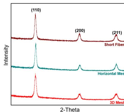
Fig. 2. XRD patterns of HEA (WTaTiCrV) composites reinforced with 9wt% of  $W_{\text{mesh}}$ ,  $W_{\text{whiskers}}$  and  $W_{3\text{D-mesh}}$ .
