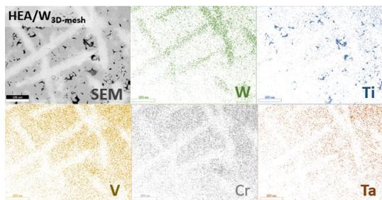
Fig. 3. Microstructure and elemental maps of  $W_{3D}$ -mesh reinforced HEA (WTaTiCrV) based composites.
