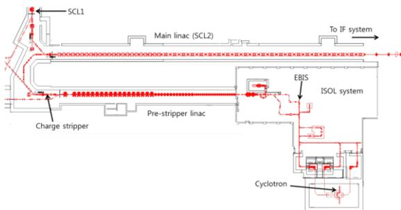
Fig.2. A layout of accelerator system of RISP.
