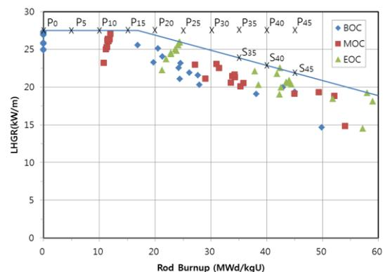
Fig. 1. Fuel rod survey data and analysis-state points.
