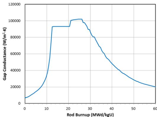
Fig. 3. Fuel rod gap conductance variation.
