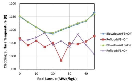
Fig. 6. PCT variation as function of fuel burnup.
