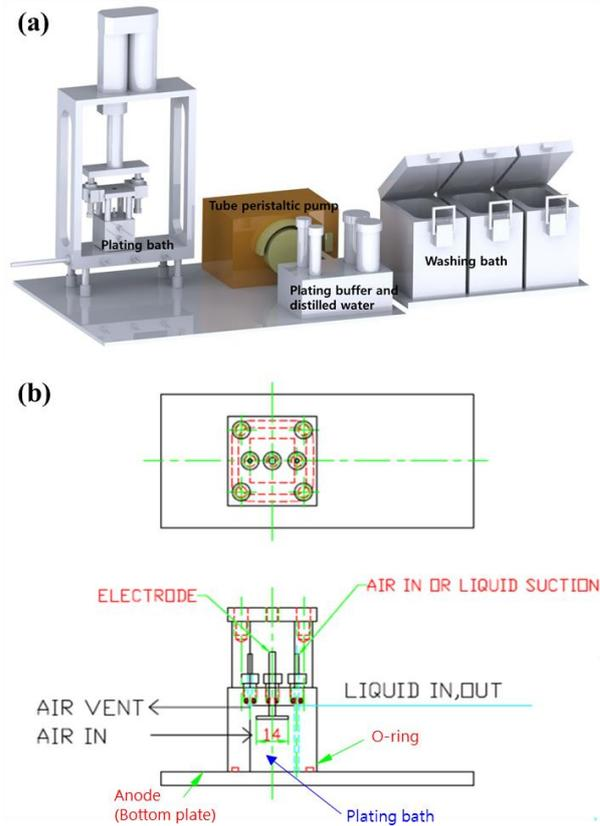
Fig. 1. A rendering image (a) and drawing image (b) of small-scale electroplating device.
