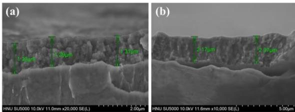
Fig. 3. SEM images for thickness of the Ni-coated Ni foil at current density of (a) 10 and (b) 20 mA/cm<sup>2</sup>.
