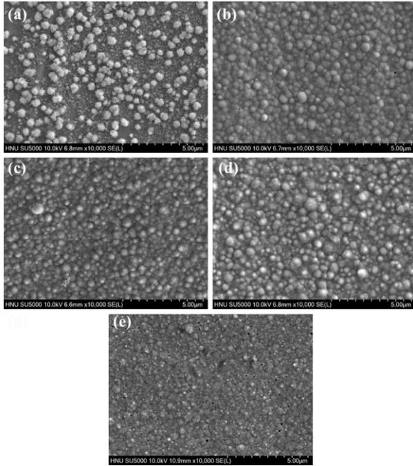
Fig. 2. Surface morphology of the Ni deposits onto Ni foil at the current density of (a) 5, (b) 10, (c) 15, (d) 20, and (e) 25 mA/cm<sup>2</sup>.
