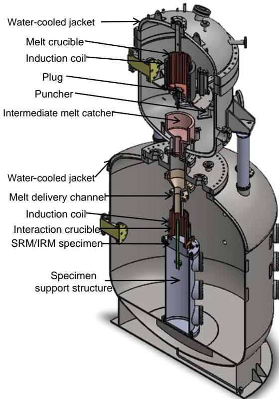
Fig. 4. Schematic of the VESTA facility.
