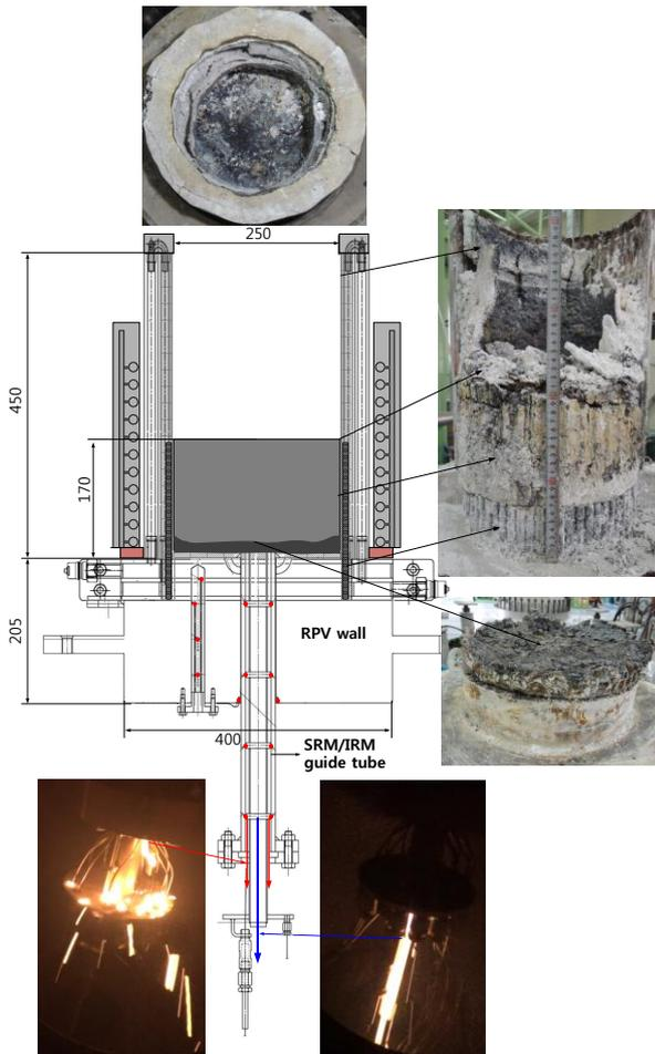
Fig. 7. Configuration of the solidified ingot in the interaction crucible and melt discharge snap shots.
