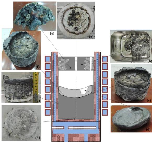
Fig. 2. Configuration of the corium ingot.
