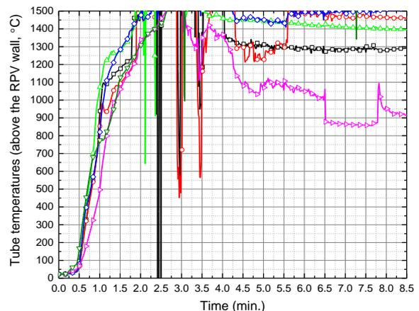
Fig. 6. Temperature distribution of the penetration tube above the RPV wall during the melt reheating process.
