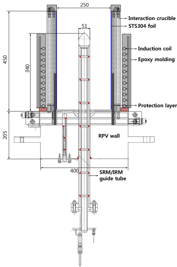
Fig. 5. Assembly of a SRM/IRM guide tube specimen and interaction crucible.
