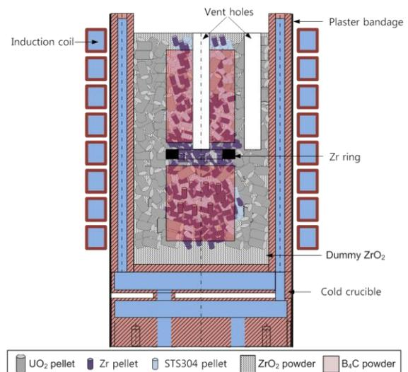
Fig. 1. Charging pattern of the melting materials.
