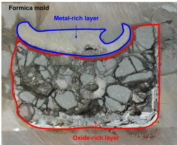
Fig. 3. Cross-sectional image of the corium ingot.
