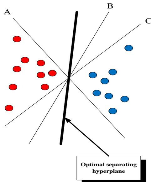
Fig. 1. Optimal separating hyperplane
