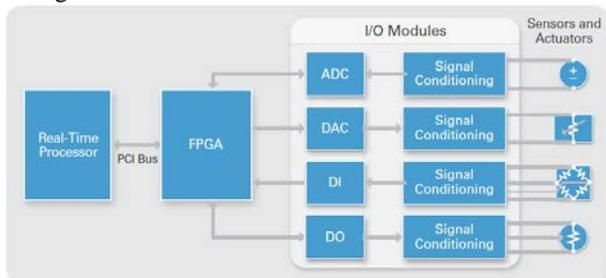
Fig. 1. Reconfiguration Embedded System Architecture.
