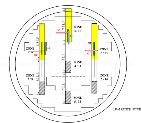
Fig. 3. LZC and ROP detectors at Zone 01, 03, and 06
