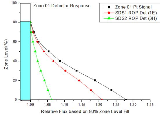
Fig. 4. LZC Pt. and ROP detectors response at zone 01
