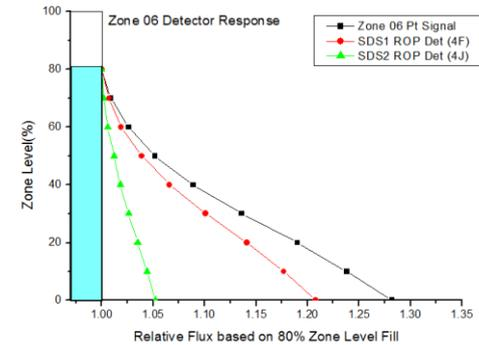
Fig. 6. LZC Pt. and ROP detectors response at zone 06
