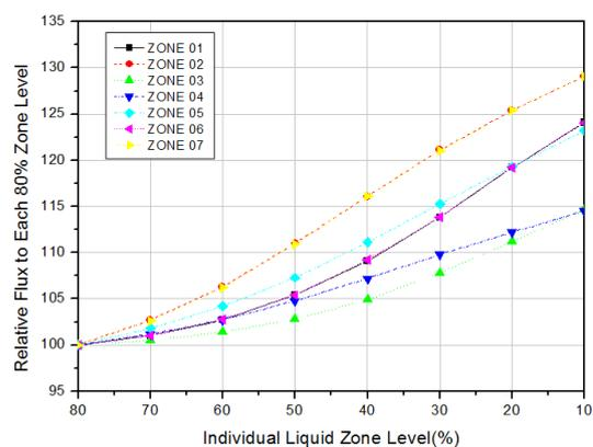
Fig. 2 Response of Each Zone Detector for Zone Drain
