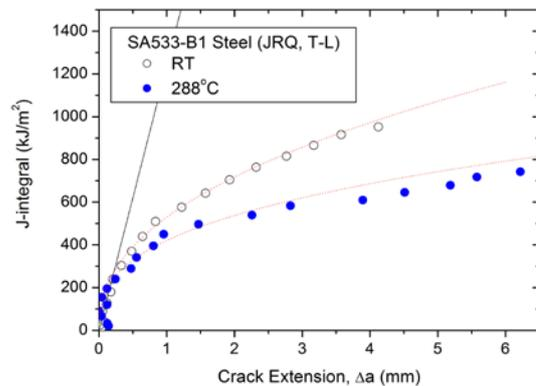
Fig. 2. J-R curves of the specimens with T-L orientation at reactor operating temperature (288°C) and room temperature.
