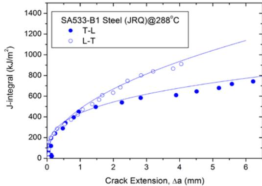
Fig. 3. A comparison of J-R curves for specimens with T-L orientation and L-T orientation taken from SA533 Gr.B-CI.1 plate, obtained at 288°C.
