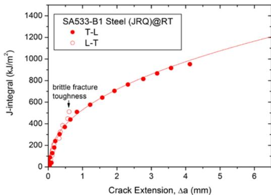
Fig. 4. A comparison of J-R curves for specimens with T-L orientation and L-T orientation taken from SA533 Gr.B-CI.1 plate, obtained at room temperature.
