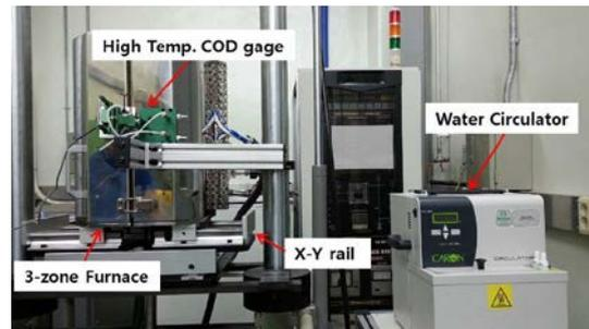
Fig. 1. Elevated temperature J-R fracture resistance testing system.
