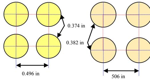
Fig. 2. Fuel rods (heater rods)
