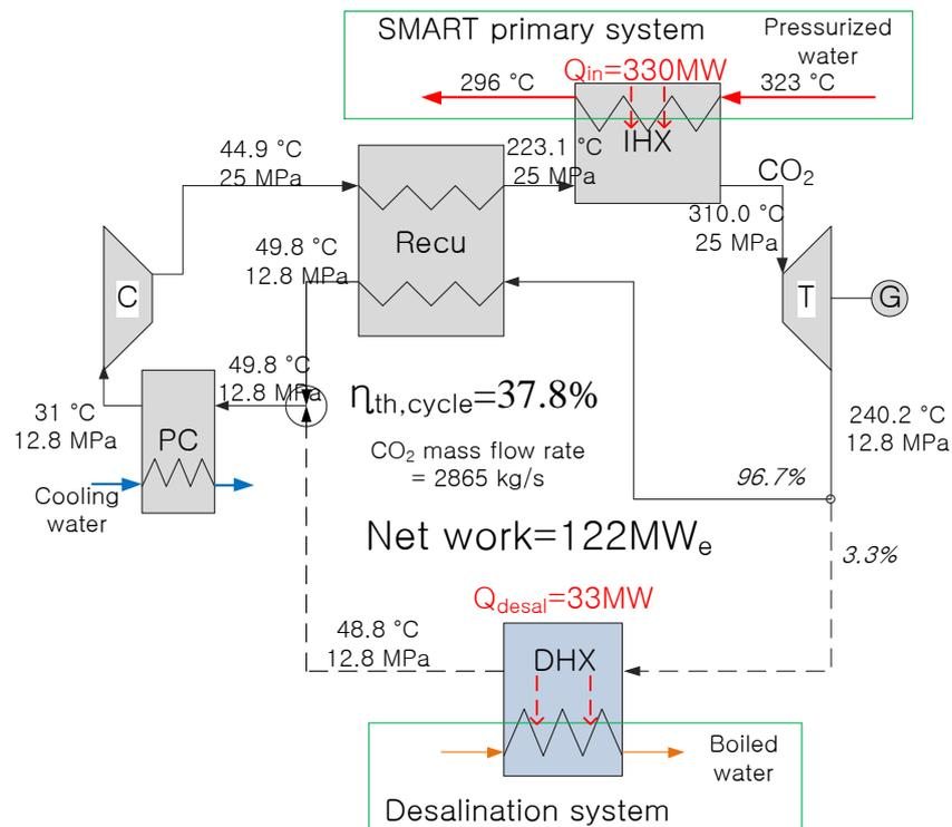
Figure 3 Cycle re-optimization results of 3rd simple recuperated S-CO<sub>2</sub> cycle
