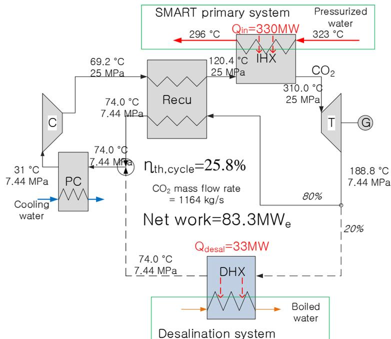
Figure 3 Results of the 3rd layout for co-generation simple recuperated S-CO<sub>2</sub> cycle
