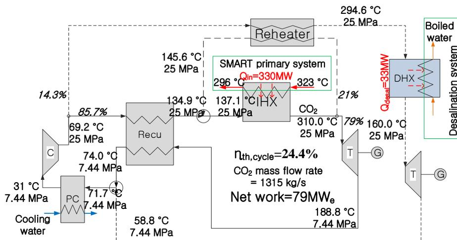
Figure 2 Results of the 2nd layout for co-generation simple recuperated S-CO<sub>2</sub> cycle
