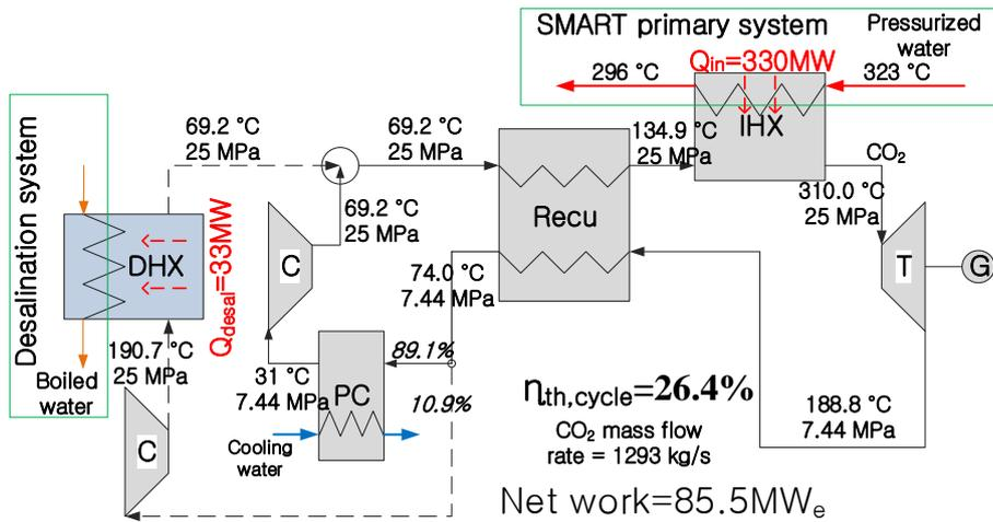
Figure 1 Results of the 1st layout for co-generation simple recuperated S-CO<sub>2</sub> cycle
